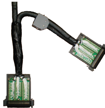
Figure 3. Cabling solution for connecting two 40-538-021 cards together also showing interconnect for instrument I/O & connection pigtail to D.U.T.
