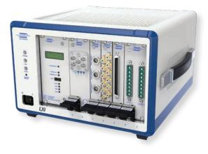
The 60-102B allows the remote operation of switching modules over long distances including world wide networks. The separation of the chassis from the controller's PCI bus simplifies system power-on sequencing and provides independence from the migration of the Windows and VISA environment.
